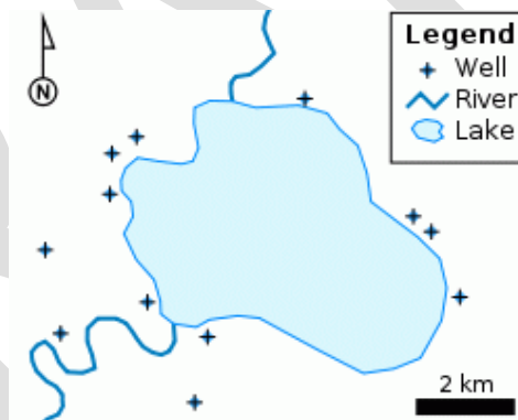
Figure 13: A simple vector map showing points for wells, lines for rivers, and a polygon for the lake (Wikimedia Commons)
